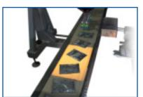
Vision System is standard on the MK-DLT pick and place system. This ensures that products do not need to come uniformly to the Delta 3 robot.
