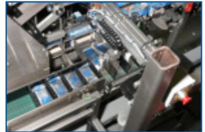
**Servopack Infeed conveyor allows the HD-LSP to reach speeds of over 350 ppm. Dual servo driven belts allow the conveyor to simultaneously load and accumulate.**
