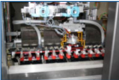
**SUBO pick, group and place end effector allows the HD-LSP to effectively collate bulk product. This unit ensures a high quality pack pattern in the carton.**
