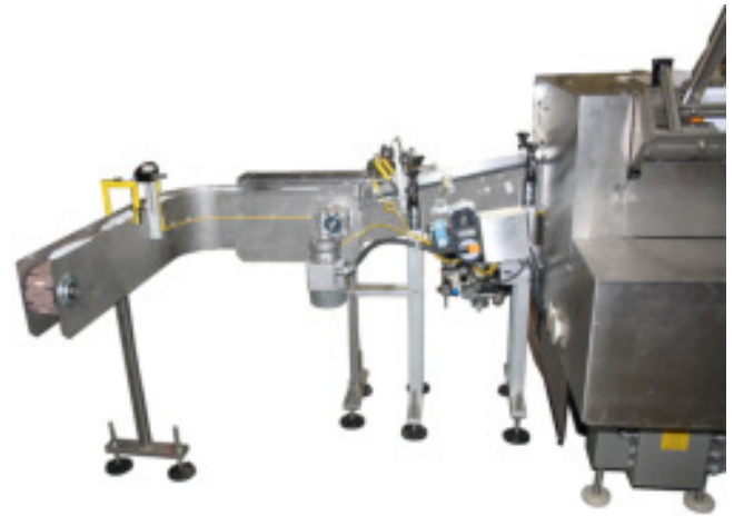
RETROFITTED CONVEYOR ON PACKAGING SYSTEM
