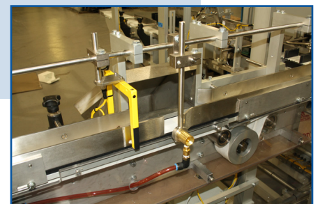
PNEUMATIC BLOWER WITH CHUTE REJECT SYSTEM INTEGRATED ON CONVEYING SYSTEM
