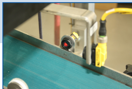
PRODUCT SENSOR ON CONVEYOR IDEAL FOR PRODUCT COUNTING AND OPEN FLAP DETECTION
