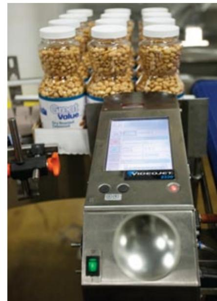
A Videojet 2330 inkjet case-coder applies product name and barcoded data onto a side of a corrugated tray loaded with plastic jars of peanuts.
