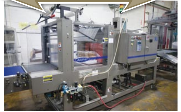
After a dozen 700-gram bottles are placed onto a finished tray, they are shrinkwrapped by a model 25TW-28 wrapper from ARPAC Group.
