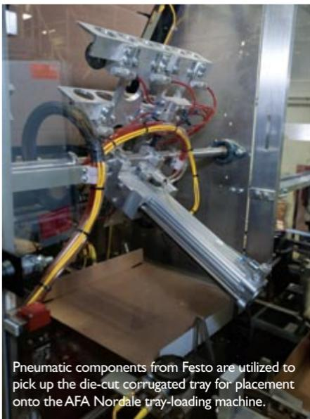
Pneumatic components from Festo are utilized to pick up the die-cut corrugated tray for placement onto the AFA Nordale tray-loading machine.
