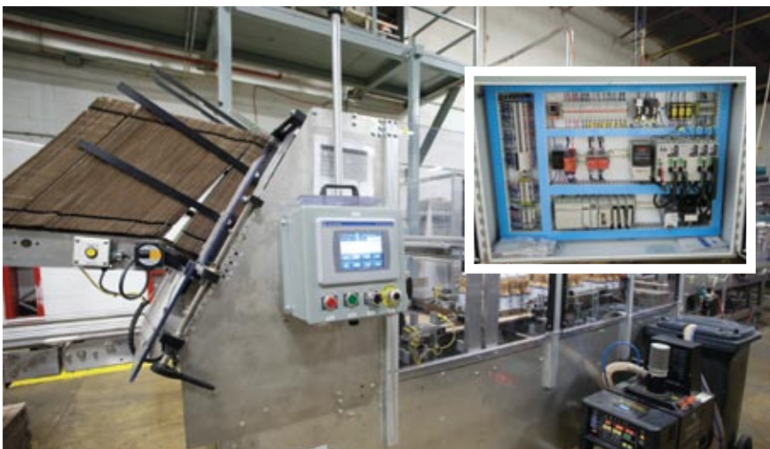
Utilizing Rockwell Automation's Allen-Bradley controls (inset), an AFA Nordale tray-loader is a key Johnvince Foods capital investment that enabled the nuts processor to reduce its secondary packaging waste.
