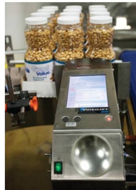
A Videojet 2330 inkjet case-coder applies product name and barcoded data onto a side of a corrugated tray loaded with plastic jars of peanuts.
