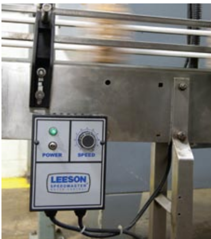
A Leeson Speedmaster controller ensures that the product on the conveyor system is always moving along the bottling line at operating optimal speeds.
