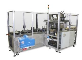
The new MK-CTP tray packer from AFA Systems provides servo driven technology for tray packing applications.
